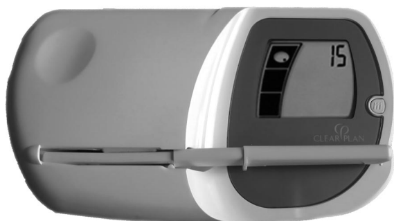
Figure 1. ClearBlue Easy Fertility Monitor with a test stick inserted. Three bars indicate low (1 bar), high (2 bars, based on detection of E3G rise), or peak fertility (3 bars and an egg symbol, based on detection of luteinizing hormone threshold).
